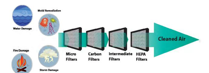
Janitized<sup>®</sup> aftermarket filters offer a variety of filter designs to maximize the efficiency of the specialized restoration equipment. From Carbon to HEPA filtration rated at 99.97% at 0.3µm; Janitized filters help improve indoor air quality during the remediation and after by capturing airborne contaminants and returning the air to a level of cleanliness equal to or better than pre-loss conditions.
